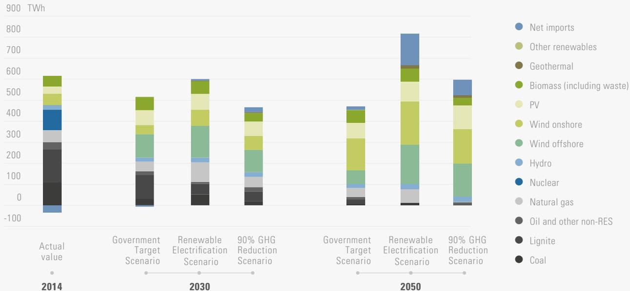
The figure refers to gross electricity generation except in the case of the 90% GHG Reduction Scenario, for which net electricity generation is shown as data for gross generation is not available.
